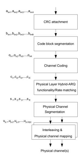
Figure 21: Transport channel processing for E-DCH
